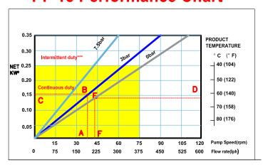
How to calculate speed/horsepower
