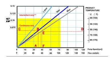
How to calculate speed/horsepower
