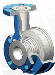
Non-metallic, lined magnetic drive pumps utilize ductile cast iron outer shell, the front casing liners shall be one single piece, transfer moulded designed with flat faced flanges, made of PFA 5mm minimum thickness.
