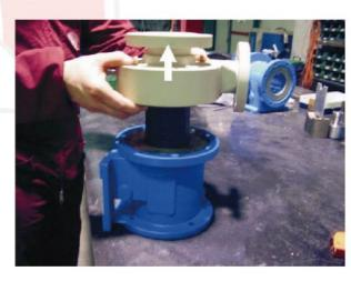
6) Pull out the internal assembly from the pump casing.
