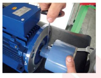
15) Using an extractor pull-out the external magnet from motor shaft.
