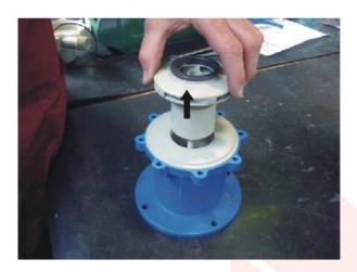
7) Pull out the rear casing with the shaft.
