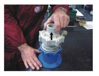
6) Pull out the internal assembly from the pump rear casing. Check status of all internal parts and replace it if necessary.
