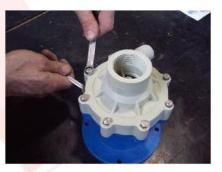
5) Pull out the pump casing and then verify the status of the O-ring and pump casing thrust bearing. Replace it if necessary.
